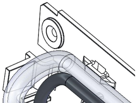
Feed Facia Kit into the AC unit cutout on right hand side of the unit.
